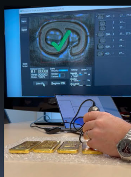
2. Gold bar verification (with USB-microscope)
